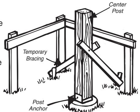
Now run a mason line from your ledger to the post, check the level with a line level and mark the post height. The height of the post should be equal to the bottom of the ledger less your beam size and desired slope (most decks are sloped slightly away from the house to encourage water to run off).
