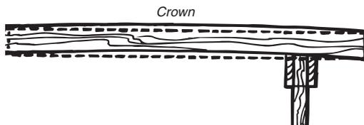
Trimming the joists to correct length can wait until you are installing the decking. This allows you to trim the deck joists to the exact length required to accept the full width of the last row of decking.
