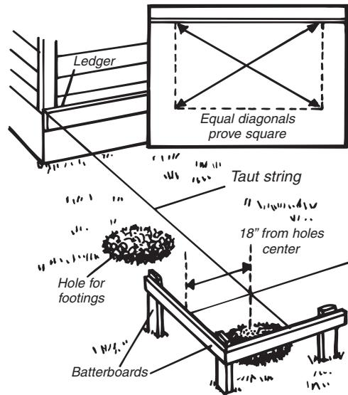
boards. Run a third string between the batter boards to establish the outside edge of your deck. Now square the deck by measuring diagonally and the moving the strings on the batter boards until the measurements are equal.
