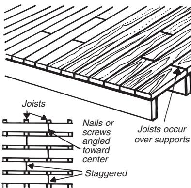
over the centre of the joist. Joints should be staggered between rows, no two joints should be adjacent to each other.
