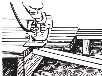
nail or carpenter pencil can be used as a spacer. Pilot holes will reduce the chance of splitting and should always be
