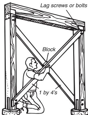
Attach the beam to the posts with appropriate hardware (See Metal Connectors) and if required by local building codes install cross bracing.
